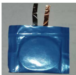
Picture of pouch cell containing Li anode, OIC-SPE electrolyte and \text{TiS}_2 cathode with binder
